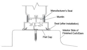
11. There will be 1/16-inch high gaps between the finish surface and the bottom of the radius wall. If the radius wall is being used as a shower wall, apply a bead of caulk along the base of the radius wall. Also apply caulk along the joints where the radius wall slides into the mounting channel and where the channel meets the finished wall. DO NOT apply sealant along the muntin bars. The blocks are completely sealed to the frame at the factory.
