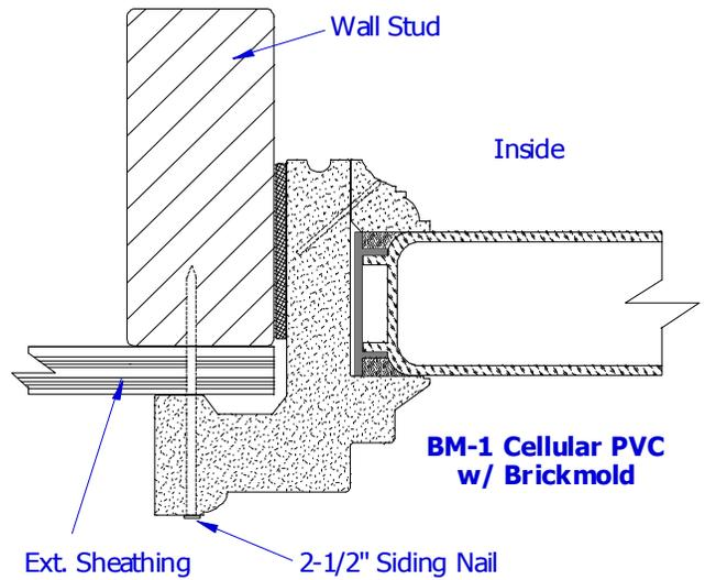
**Note: We strongly recommend the use of flashing and/or flashing tapes and sill pans as stated in ASTM E 2112-01. However, due to variation in codes and building types, it is left up to the end user to determine the proper installation of these items.**
