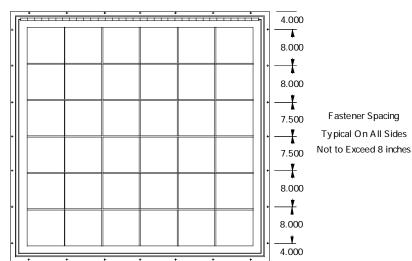
Fastener Spacing Typical On All Sides
